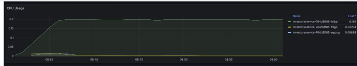
Figure 6.4: CPU usage of the InventoryService pod during the 30-minute load test, showing sustained maximum utilization.
